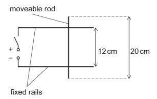
The whole arrangement is placed in a uniform magnetic field of magnitude 0.50 T that is directed perpendicularly into the page.
