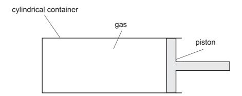
The particles of the gas are moving with an average speed v, and collide with the surface of the piston with a frequency f.
