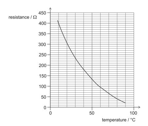
When the temperature of the thermistor is 10 °C the current in the circuit is 25 mA.
