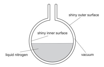
The vessel has a double wall made from a poor thermal conductor. There is a vacuum in the gap between the two walls.
